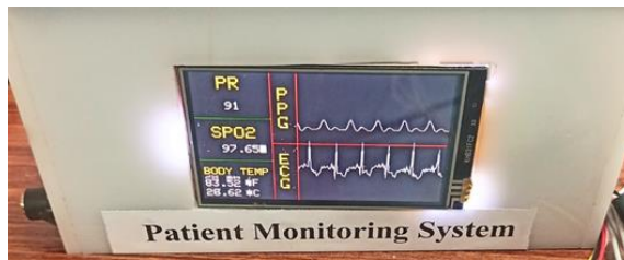
Figure 15. The Patient Monitoring System displays real-time vital signs, including Pulse Rate (PR), SpO2, Body Temperature, and Electrocardiogram (ECG) readings on an LCD screen.
