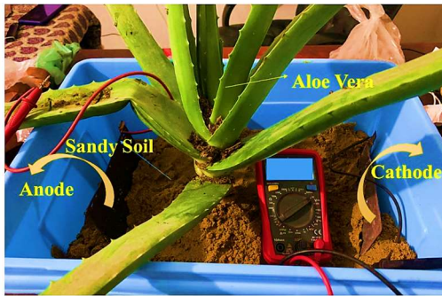
Figure 6: Simple plant setup
