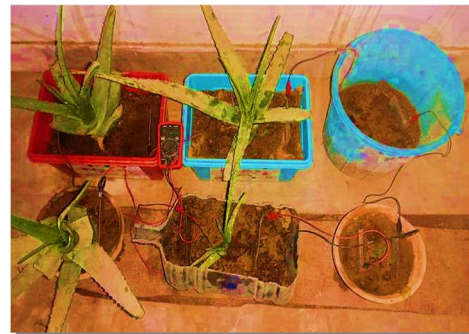
Figure 7: Setup to investigate Series Connection
