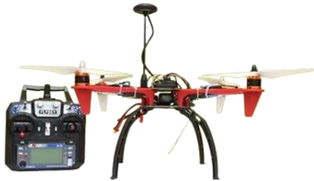
Figure 4: Custom F450 Quadcopter System with Remote Controller [31]
