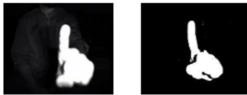
Figure 4: Background subtraction on Microsoft Kinect's depth camera's image
