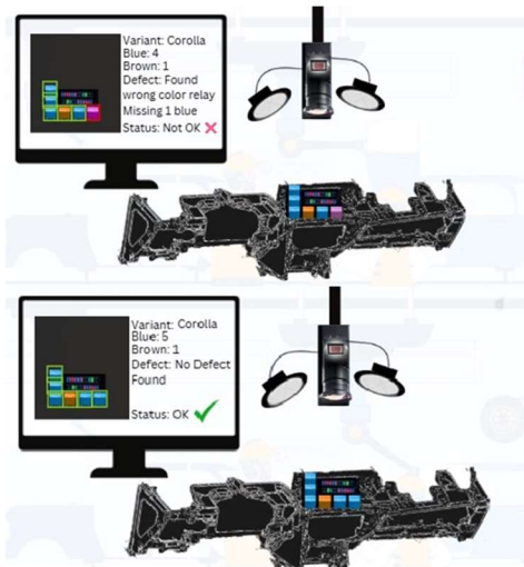
Figure 13: Schematic diagram of the Detect-iPro system architecture
