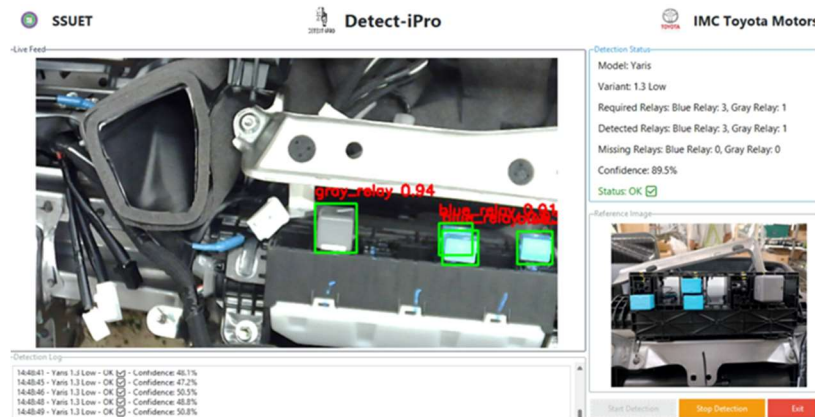
Figure 14: GUI output for relay box inspection with bounding boxes and defect classification
