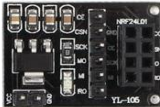
Figure 9: nRF24L01 Breakout Adapter with Voltage Regulator
